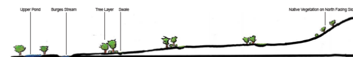
Figure 5.19 Section E-E' Swales appear on contour at intervals greater than 30 meters intercepting surface flow and allowing for the reestablishment of perennial vegetation on the downslope side of swales. Total section length = 300 meters. Elevation change from high point to low point = 34 meters.
