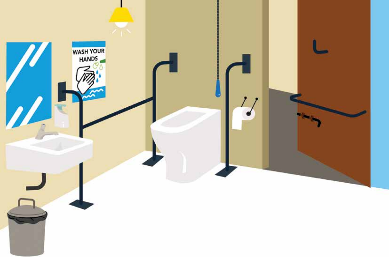
Figure 4: An example of the interior of a female-friendly and accessible cubicle.
