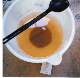
Floc formation after PUR addition
