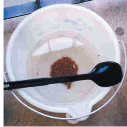
Floc formation after complete stirring
