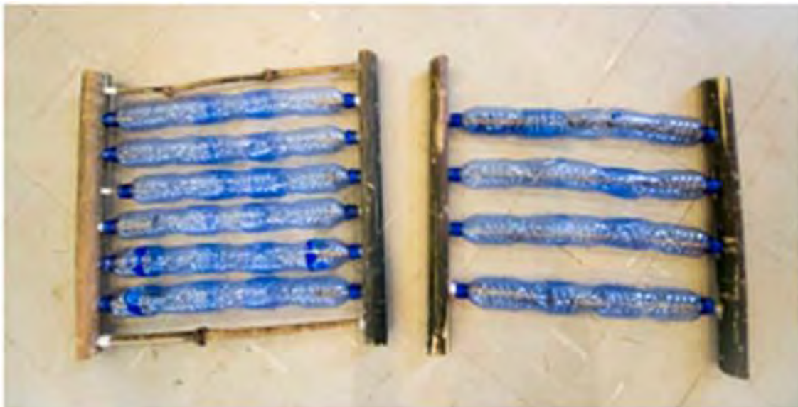
Figure 14. Initial PET bottle wall mode (right); second iteration with horizontal bars on top/bottom for added stability (left)
