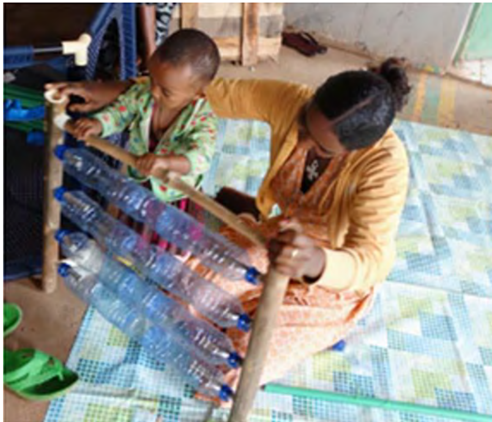
Figure 15. Sixteen-month old playing with and testing the first iteration of the PET bottle sidewall
