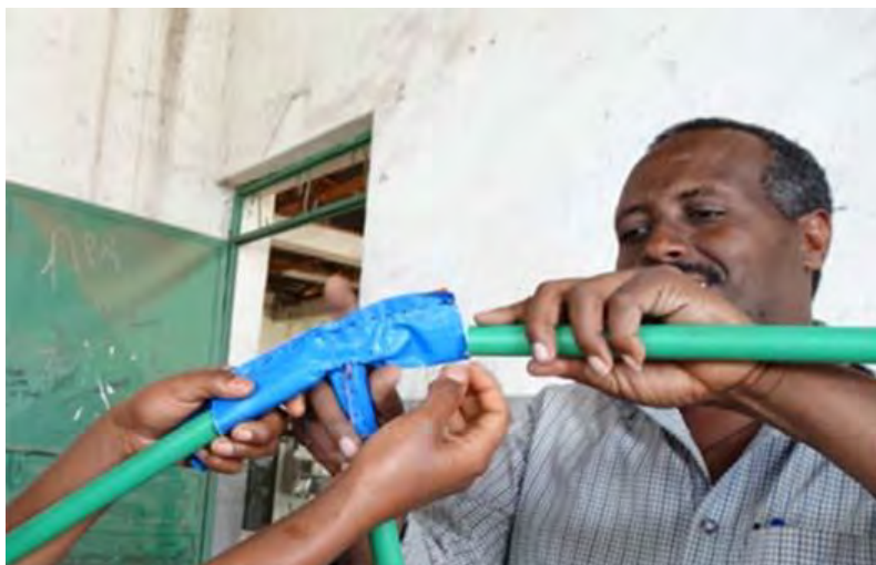
Figure 8. Tarp joint produced in the first iteration. Later substituted for welded metal joint
